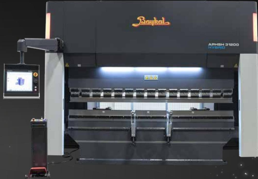
The Hydraulic system are directly connected to two small oil tanks. The advantage is that the cnc press brake is more precise and is not affected by temperature variation, as opposed to traditional machines.
